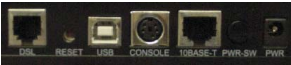
Figure 3 View of back of Frontier DSL modem
